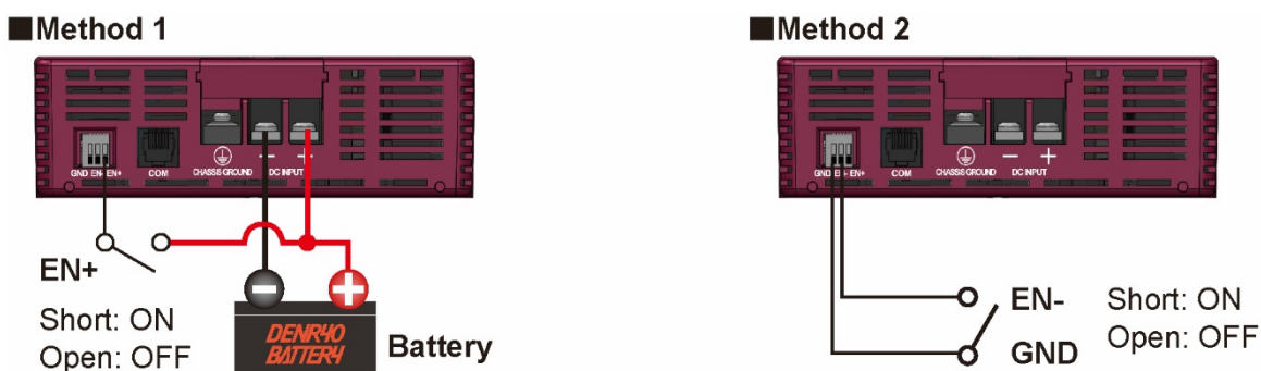
Figure 5.4 The wiring of remote connector
