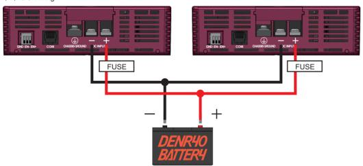
①Connect each DC input terminal (+) and connect each DC input terminal (-) in a junction box respectively (\*4 \*5). Connect the grounding terminal to earth ground if necessary.
