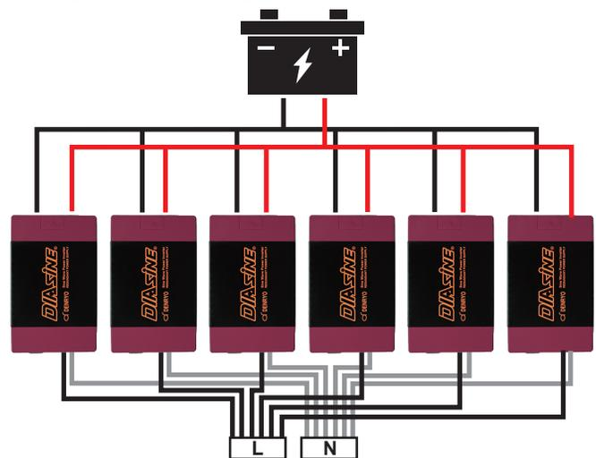
Connect the load's L and N to the coupled L and N cables.
